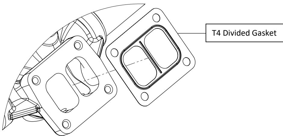
**After installation, drive the vehicle for approximately 100 miles then, while the vehicle is warm re-torque all the bolts and clamps, as the bolts sometimes loosen up after being heated and cooled a few times.**
